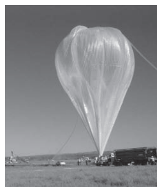
Figure 2.17 Much of what we know about muons in cosmic rays was learned from balloon flights carrying sophisticated detectors. This balloon is being prepared for launch in NASA's Ultra Long Duration Balloon program for a mission that may last up to 100 days. The payload will hang many meters below the balloon. Victor Hess began the first such balloon flights in 1912 (when he discovered cosmic rays), and much improved versions are still launched today from all over the world to study cosmic rays, the atmosphere, the sun, and the universe.
